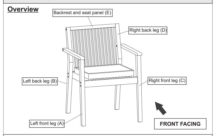
This Chair has multiple parts and may require up to 30 minutes to assemble. To give you an overview of the Chair parts, the above picture is to help you put the various parts into perspective. Please read through the instructions below to familiarise yourself with the parts and steps before assembly.
