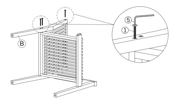
Secure the Left back leg (B) onto the Backrest and Seat panel (E) using Screw (1) and the Allen Wrench (5).
