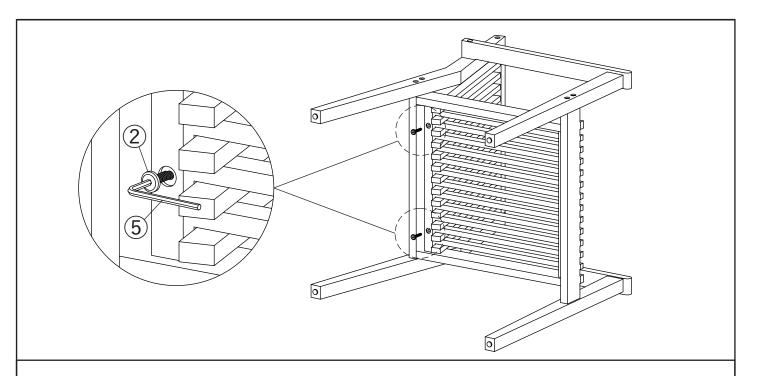
Secure the Seat panel and Back panel using Screw (2) and the Allen Wrench (5). **DO NOT fully tighten the Screw at this time.**
