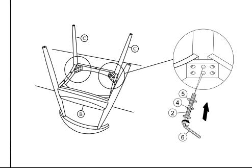
Attach Front Legs(C) to Seat(B) using Bolts(2), Spring Washers(4), and Washers(5) with Allen Key(6) as pictured above.
