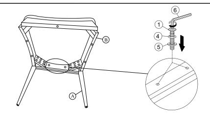
Attach Chair Seat(B) to Back Rest(A) using Bolt(①), Spring Washer(④), and Washer(⑤) with Allen Key(⑥). Do not fully tighten the Bolts.
