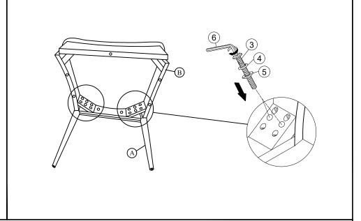
Attach Chair Seat(B) to Back Rest(A) using Bolts(③), Spring Washers(④), and Washers(⑤) with Allen Key(⑥). Do not fully tighten the Bolts.
