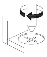
**EN**\_Turn cam lock clockwise to tighten.
