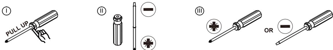
Screwdrivers can be converted to Phillips and Slotted.
