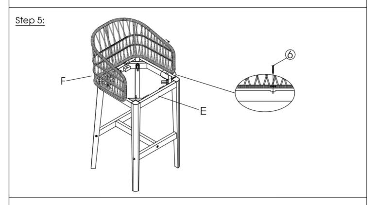
Fix the backrest (F) with Seat Panel Frame (E) by using 04 Screws (6) by screwdriver DO NOT fully tighten the screws.
