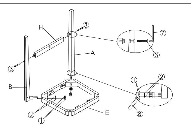
With the help of your adult partner, place the Seat Panel Frame (E) facing down and then add the Front Right Leg (A) and Front Left Leg (B) to the Seat Panel Frame (E) and secure by using Nuts (1) + washer (2) by Wrench (8) after that fix the Front Connecting Bar (H) with 02 screws (3) by Allen Wrench (7). **DO NOT fully tighten the Nuts and screws**.
