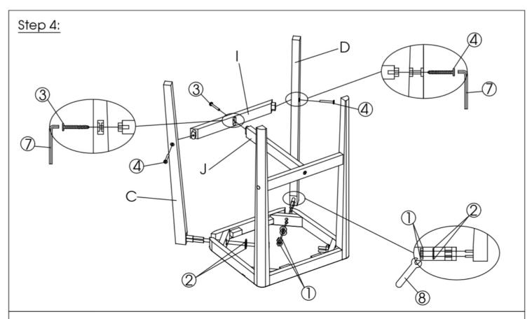
Add the Back Left Leg (D) and Back Right Leg (C) to the Seat Panel Frame (E) and secure by using Nuts (1) + washer (2) by Wrench (8). Fix the Back Connecting Bar (I) with 02 screws (4) by Allen Wrench (7) after that fix the Back Leg Frame with the cross Bar (J) by Screw (3) and the Allen Wrench (7). **DO NOT fully tighten the Nuts and screws**.
