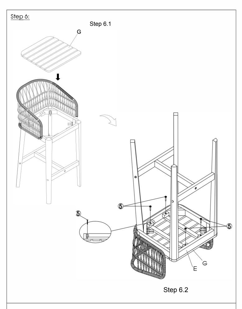
Fix the Seat Panel (G) with Seat Panel Frame (E) by using 04 Screws (5) by screwdriver. **DO NOT fully tighten the screws**.
