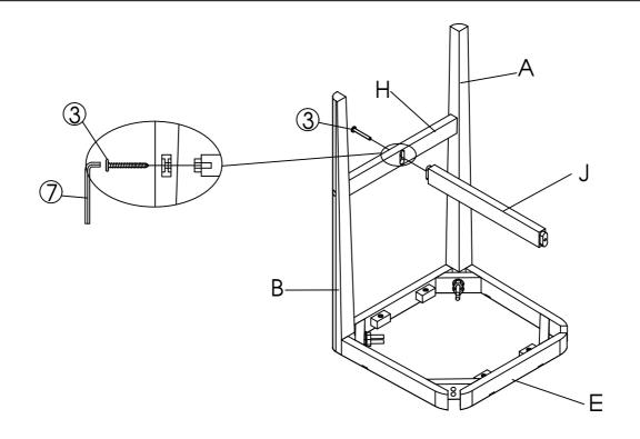
Fix the Cross Bar (J) with the Front Connecting Bar (H) by using 01 screws (3) by Allen Wrench (7). **DO NOT fully tighten the screws**.
