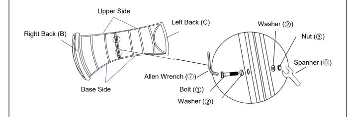
Place the Right Back(B) and Left Back(C) on a clean, non-marring surface. Attach Right Back(B) to Left Back(C) using Bolts(①), and Washers(②) on one side and Washers(②) and Nuts(③) on the other side, with Allen Wrench(⑦) and Spanner(⑥).
