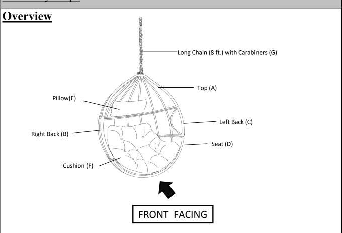
This Basket has multiple parts and may require up to 30 minutes to assemble. The above picture is to help you put the various parts into perspective. Please read through the instructions below to familiarize yourself with the parts and steps before assembly.
