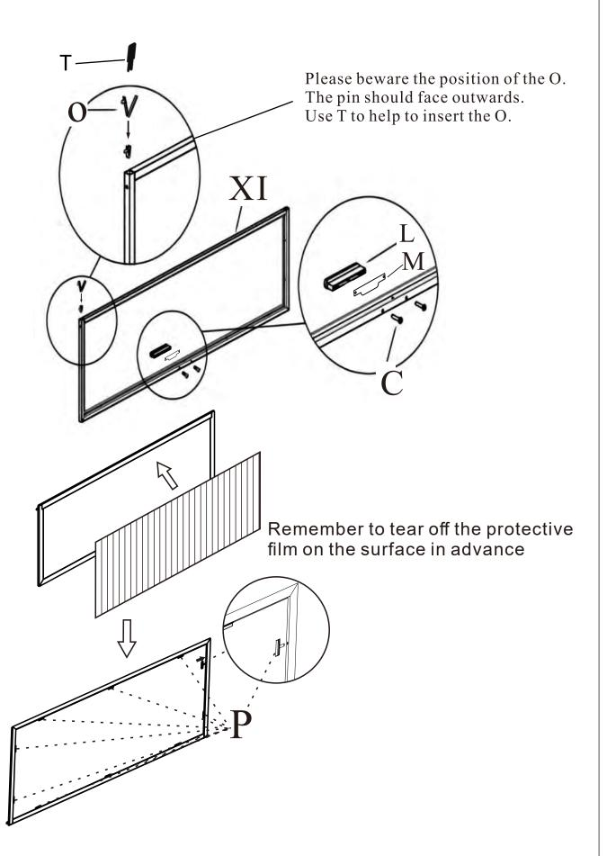
Press the assembled O to install XI & XII to the cabinet body. Install Q for shelf. Make sure clips in 4 corners are at the same height.
