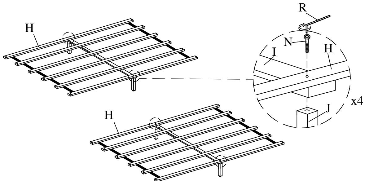
8 Tighten JCBB Bolt (K) on the Headboard Leg (E) and Footboard (B) with the Allen Key (S). Then, attach the Slat (H) to the Side Rail (C & D) using CSK Screw (O) with a screwdriver (not provided). The distance of the slats should be sufficient to obtain desirable bed stability.
