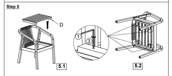
5.1) Position Seat Panel (D) to the assembled part in Step 4 as shown above picture.5.2) Attach Seat Panel (D) to Left Leg Panel (A) and Right Leg Panel (B) by using 4
