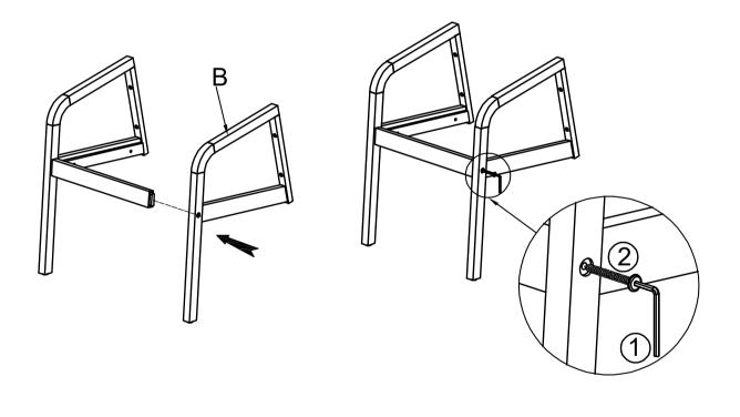
With assistance from your adult partner, attach Right Leg Panel (B) to Front Bar (E) by using Screw (②) and Allen Wrench (①) to secure as shown above.
