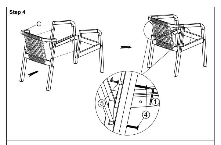
With assistance from your adult partner, attach Backrest Panel (C) to Left Leg Panel (A) and Right Leg Panel (B) by using 4 Bolts (4) and 4 Sleeve nuts (5) and 2 Allen Wrench (1) to secure as shown above.
