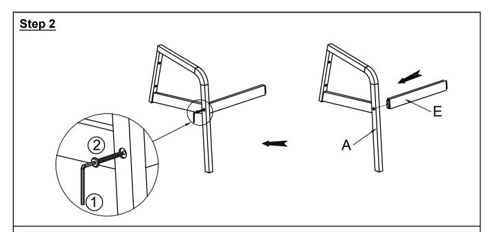
With assistance from you adult partner, attach Front Bar (E) to Left Leg Panel (A) by using Screw (②) and Allen Wrench (①) to secure as shown above. **Do not fully tighten the Screws.**
