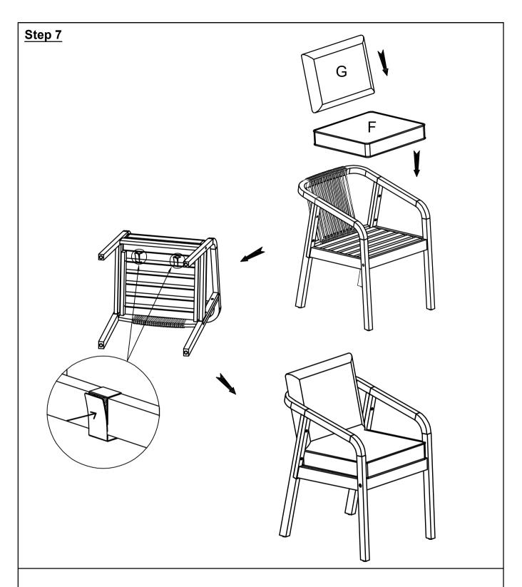
Place Seat Cushion (F) onto the Chair. Tie the magic tape straps of Seat Cushion (F) to the slats of Seat Panel (D) as shown above.
