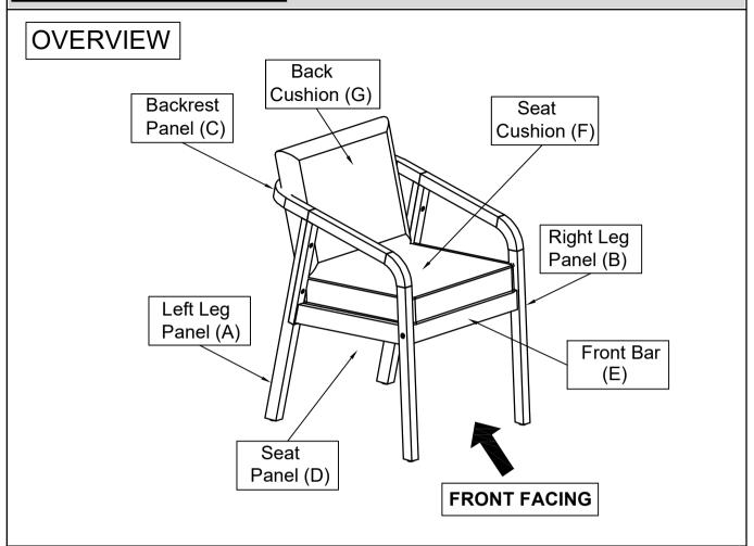
This Chair has multiple parts and may require up to some 30 minutes to assemble. To give you an overview of the Chair, the above picture is to help you put the various parts into perspective. Please read through the instructions here below to familiarise the parts and steps before assembly.
