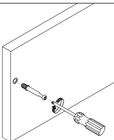
The base of the Cam Screw should be flush with the panel
