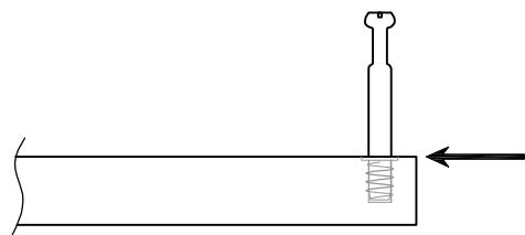
Screw the Cam Screw into the prethreaded hole. Tighten with a screwdriver until snug.
