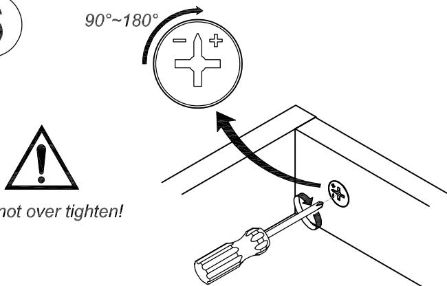
Using a screwdriver, turn the Cam Lock at least 90° clock-wise to lock the two panels firmly together.
