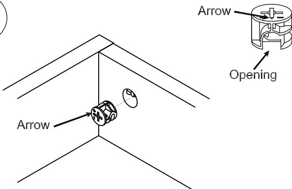
Insert the Cam Lock into the large hole. Make sure the arrow and the opening in the Cam Lock are facing the Cam Screw.
