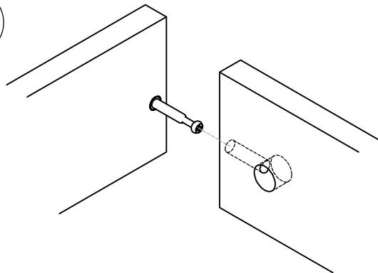
Connect the panels. Insert the Cam Screw into the small hole in the adjoining panel.
