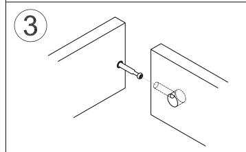
Connect the panels. Insert the Cam Screw into the small hole in the adjoining panel.
