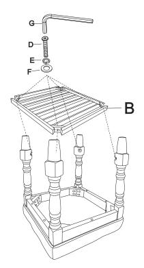
Step 3: Install as instructed on the label, Use Part D (screw), Part E (ring), Part F(Gasket), connect Part B(bottoms) to Part C(leg), and tighten with Part G.
