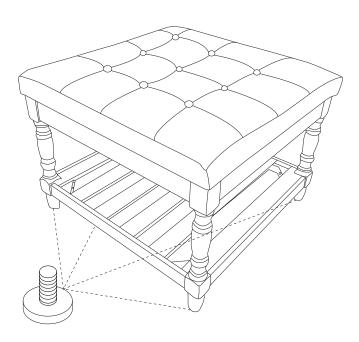
Step 4: Finally, install Part H(footpad) on Part C(leg)
