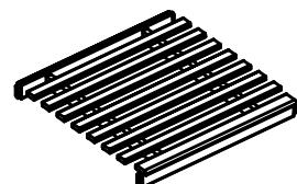
A line drawing of the seat, which is a rectangular frame with a series of horizontal slats. |
