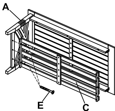
Attach tray table (C) to the leg frame (A) secure using 1" bolts (E).
