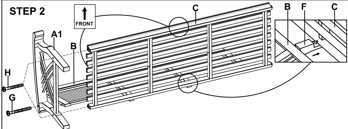
Attach back support (B) and seat (C) into right side frame (A1), secure using 3 1/2" bolts (G) and 2" Bolts (H), as shown. Tighten all bolts using screwdriver.
