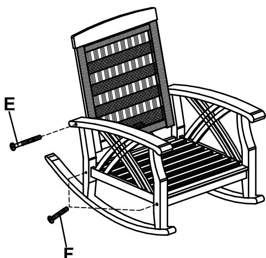
Upright the rocker and repeat the same procedure in step 2 to secure right side frame (A1) using 3 1/2" bolt (E) and 2" bolts (F). As shown. Tighten all bolts and screw using screwdriver.
