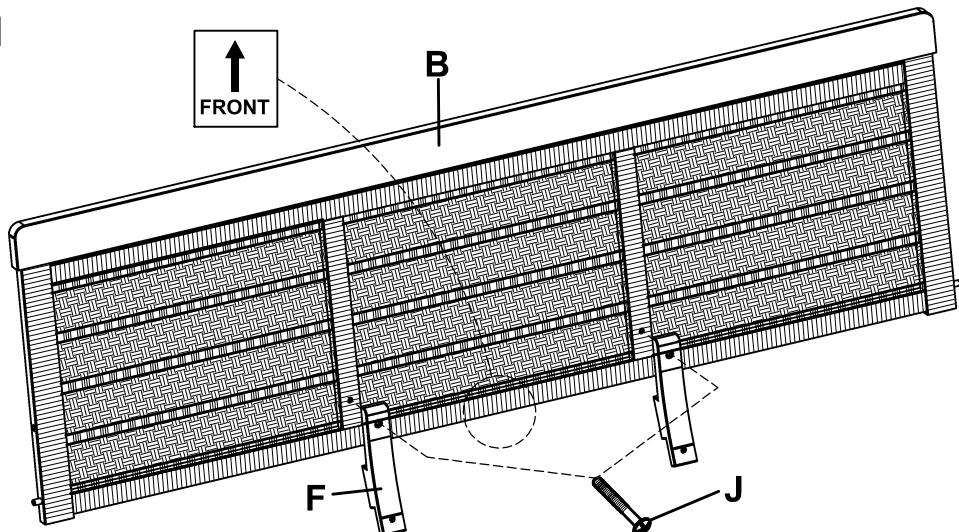
Attach back support (B) and back support holder (F), secure using 1 1/4" bolt (J), as shown. Tighten all bolts using screwdriver.
