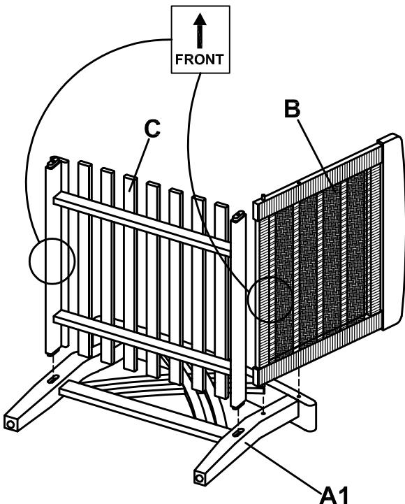
Attach back support (B) and seat (C) into right side frame (A1)
