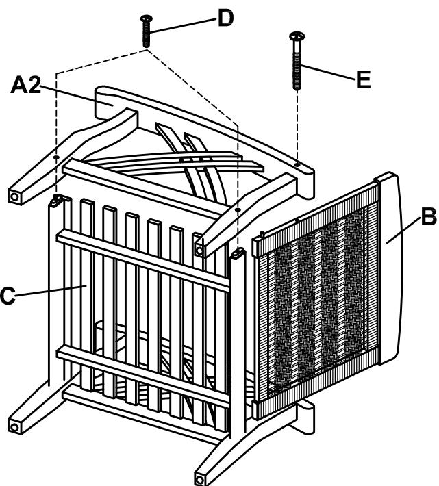
Attach left side frame (A2) to the assembly from step 1, secure using 2" bolts (D) and 3 1/2" bolt (E), as shown. Tighten all bolts using screwdriver.
