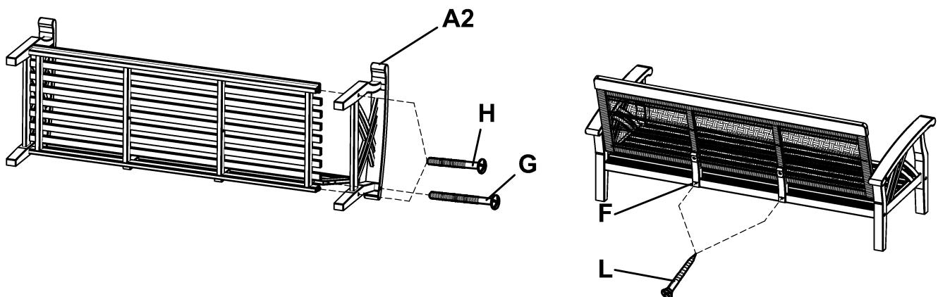
Attach left side frame (A2) into pre-assembled frame, secure using 3 1/2" bolts (G) and 2" Bolts (H). Attach back support holder (F) and seat (C) secure using 1" screw (L) as shown. Tighten all bolts and screws using screwdriver.
