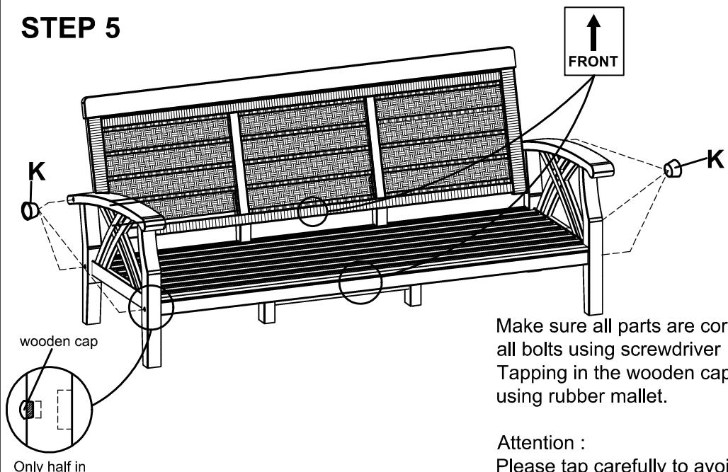
Make sure all parts are correctly connected and tighten all bolts using screwdriver .
