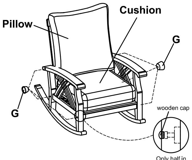
Make sure all parts are correctly connected and tighten all bolts using screwdriver. Tapping in the wooden caps (G) to cover bolts head using rubber mallet.
