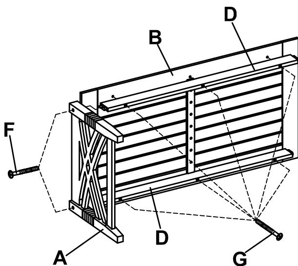
Attach apron (D) into top table (B). Secure using 2 3/4" bolts (G), then attach into leg frame (A). Secure using 1 3/4" bolts (F). Tighten all bolts using screwdriver.
