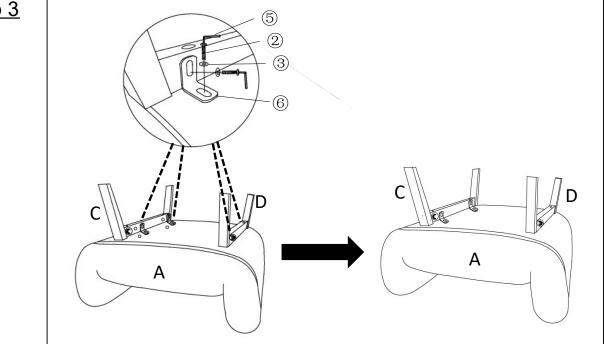
Place the Angle Irons(⑥) on the side of the Wooden Legs(C&D) and align it with the installation position.
