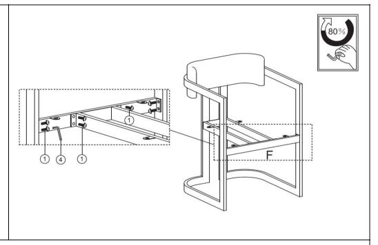
Attach Connection (F) to assembled Frame using the Bolt (1) with Allen Wrench (4) as shown above.
