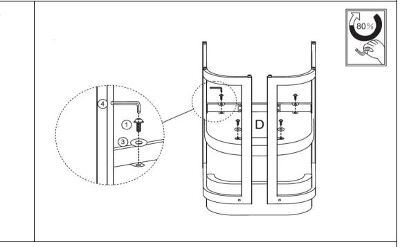
Put the chair bottom up. Attach Seat Cushion(D) to assembled Frame using the Bolt (1) and Washer (3) with Allen Wrench (4) as shown above.
