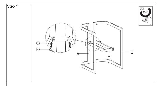
Attach the Connection (E) to Left Leg Frame(A) and Left Leg Frame(B) using the Bolt (①) with Allen Wrench (④) as shown above.
