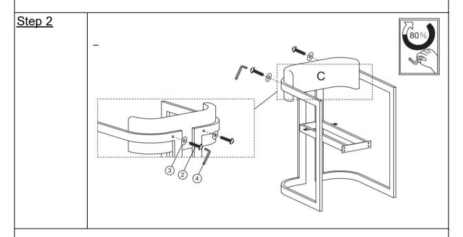
Attach Back(C) to assembled Leg Frame using the Washer (③) and Bolt (②) with Allen Wrench (④) as shown above.
