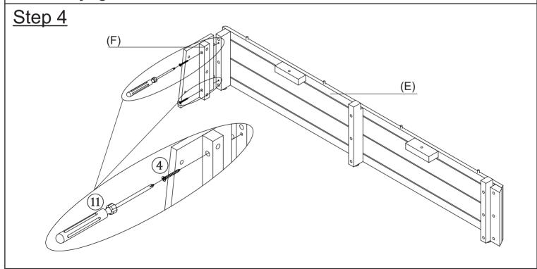
Attach the Right Side Stretcher (Right Loveseat) (F) to the Front Stretcher (Right Loveseat) (E) using Screw (4) and the Screwdriver (11) as shown above.
