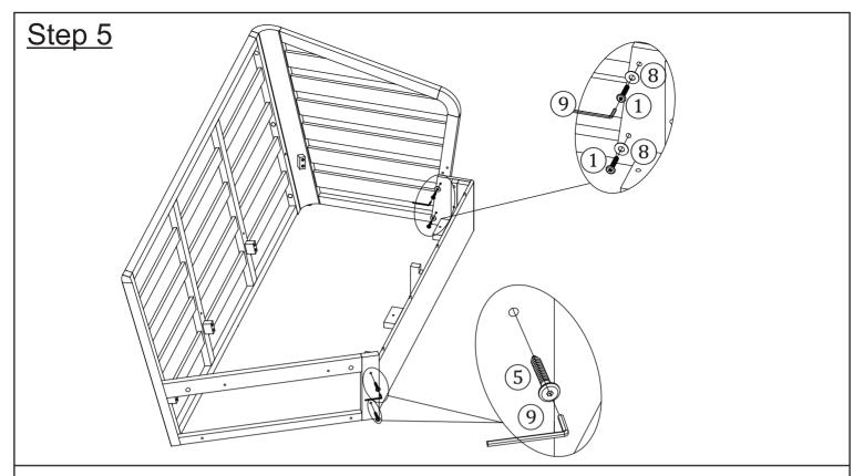
Attach Step 4 to Step 3 using Bolts ①, Washer ⑧, Screws ⑤ and the Allen Wrench ⑨ as shown above.
