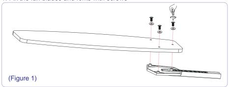
2: Assemble the blade assembly with the screws provided.
