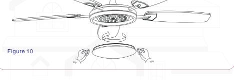
Installation is now finished . Turn on the power switch. Then the fan lights are on Test and pair your fan immediately using the remote control
