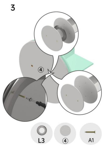
Align the large holes in the turntable with the large holes in the ④ board, then screw the small screws into the small holes to lock them in place
