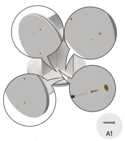
Reverse the chassis and align the two boards Rotate the turntable and find the small holes at the large holes to screw in the screws
