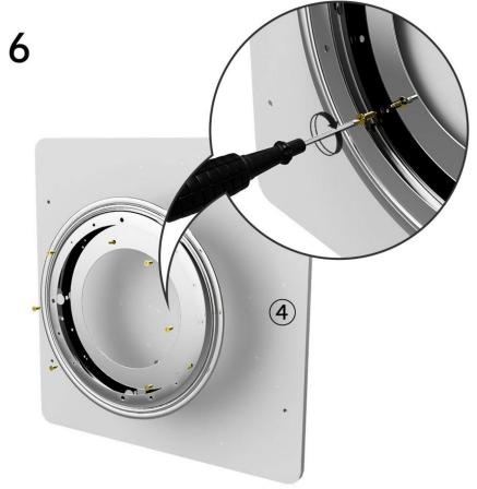
Align the large holes in the turntable with the large holes in the ④ board, then screw the small screws into the small holes to lock them in place
