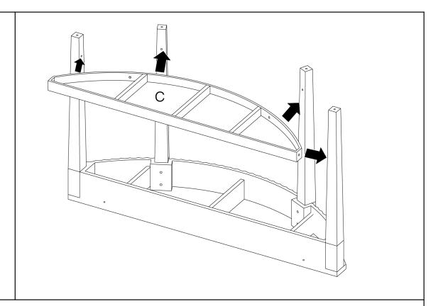
Align shelf board (C) with the pre-drilled holes on the 4 legs.
