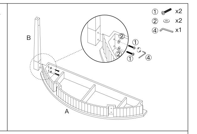
Attach legs(B) to top board(A) with hex bolt(1) and flat washer(2)
