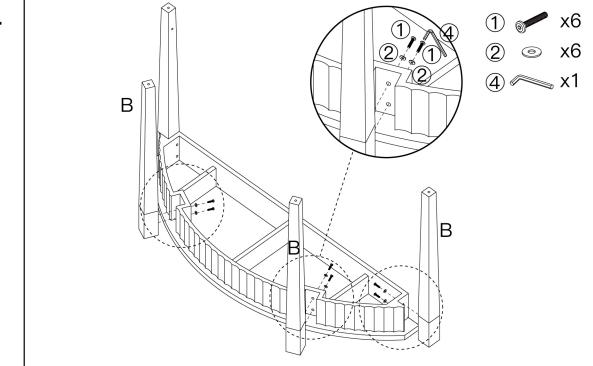
Follow step 1, attach the rest 3 legs(B) to top board (A) with hex bolt(1) and flat washer(2)
