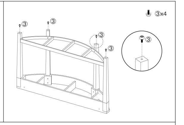
Screw adjustable leveling glide (3) on the legs(B).
