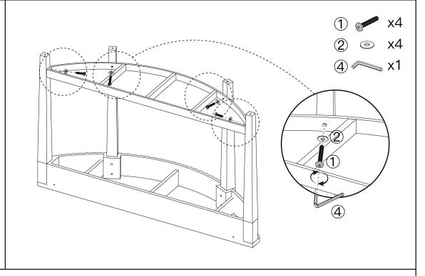
Attach shelf board (C) to legs (B) with hex bolt (1) and flat washer((2)).
