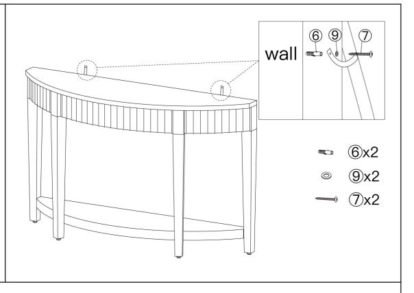
Drill holes on the wall, insert expansion plugs(6) into the holes, align with the expansion plugs (6), install the Anti-Tipping webbing (5) with long screw (7) and flat washer (9).
