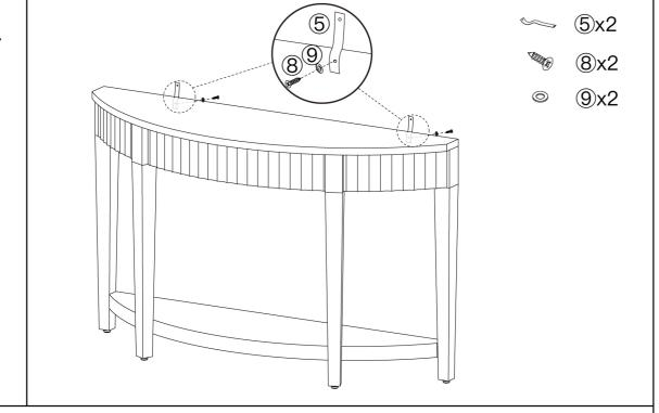
Align with the pre-drilled hole on back of the top board(A) ,install the Anti-Tipping webbing (5) on on back of the top board (A) with short screw (8) and washer (9).
