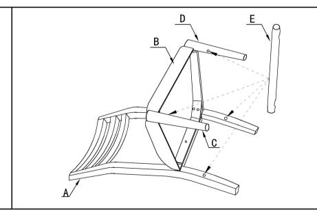
Connect the Connecting Rod(E) to Chair Back(A) & Left Leg(D), Chair Back(A) & Right Leg(C), Right Leg(C) & Left Leg(D) as shown above.
