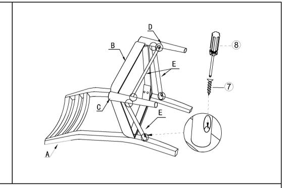
Use the Screwdriver ( $\otimes$ ) and Screws ( $\bigcirc$ ) to affix the Connecting rods (E), as shown in the picture above.
