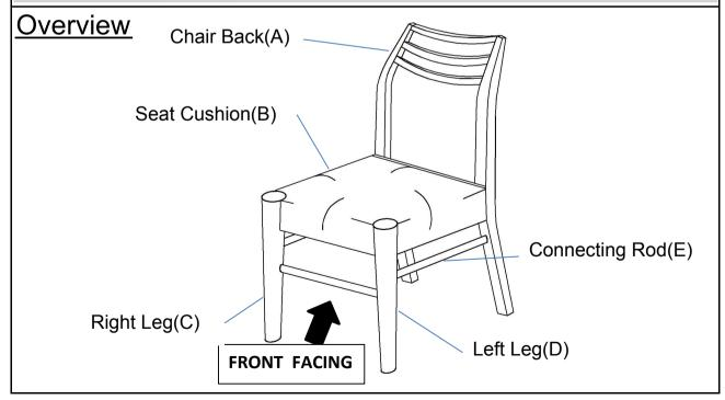
This Chair has multiple parts and may require up to some 30 minutes to assemble. To give you an overview of the chair parts, the above picture is to help you put the various parts into perspective. Please read through the instructions below to familiarise yourself with the parts and steps before assembly.
