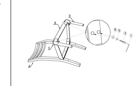
Install the Right Leg (C) and Left Leg(D) using the Allen Wrench (①), Bolts (③), Spring washers (⑤) and Flat washers (⑥), as pictured above.
