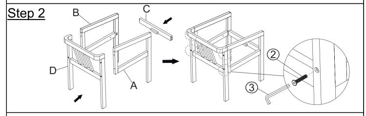
**2**.Place the Left Leg Panel (A) and Right Leg Panel (B) upright as shown in the picture above onto aclean, soft surface to avoid any scratches or damages to the product.
