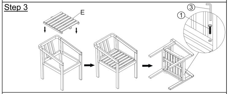
**3**.Attach the Seat Panel (E) into the Chair as shown in picture above. Affix the Seat Panel (E) to the Chair using Bolts (1) and the Allen Wrench (3).
