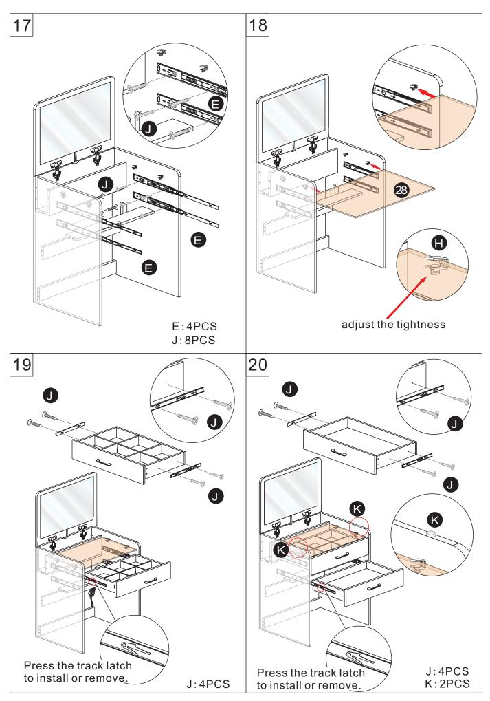
Notice: Install relevant screws, don't tighten completely at beginning Alignment & Tighten fully when you complete the seat base section.
