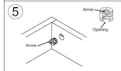
Insert the Cam Lock into the large hole.
