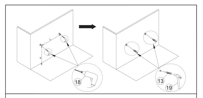
B: Affix the Plastic Anchor to the wall Using a Power Drill(18)(not provided), drill a hole on the wall, then insert a Plastic Anchor (13) into the hole using a Hammer(19) (not provided). Repeat this step to affix the other Plastic Anchor (13) into the wall, as shown above.
