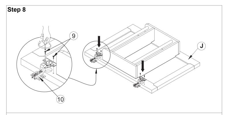
Insert Hinges (10) and Right door (J) with Screws M4x15 (9).
