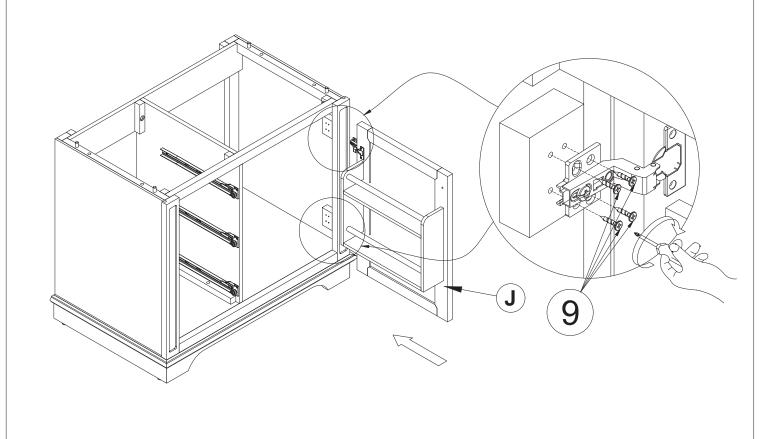
Insert Right door (J) and Step 7 with Screws M4x15 (9).
