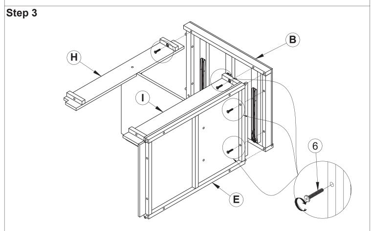
Insert Left side frame (B), Bottom frame (E), Rear top bar (H) and Rear bottom bar (I) with Bolt M6x30 (6).
