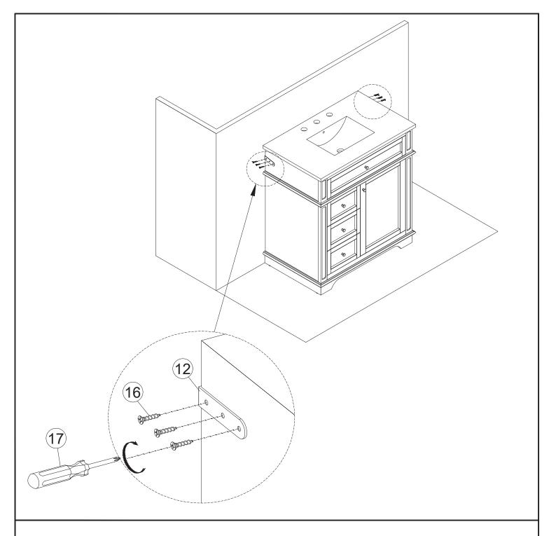
D: Move the Vanity against the wall. Then connect the L-shaped Metal Bracket (12) to Vanity position on the wall by using the Self Tapping Screws (16) and Screwdriver (17)(not provided), as shown above. The Vanity Restraint Device is now installed and is ready for use.
