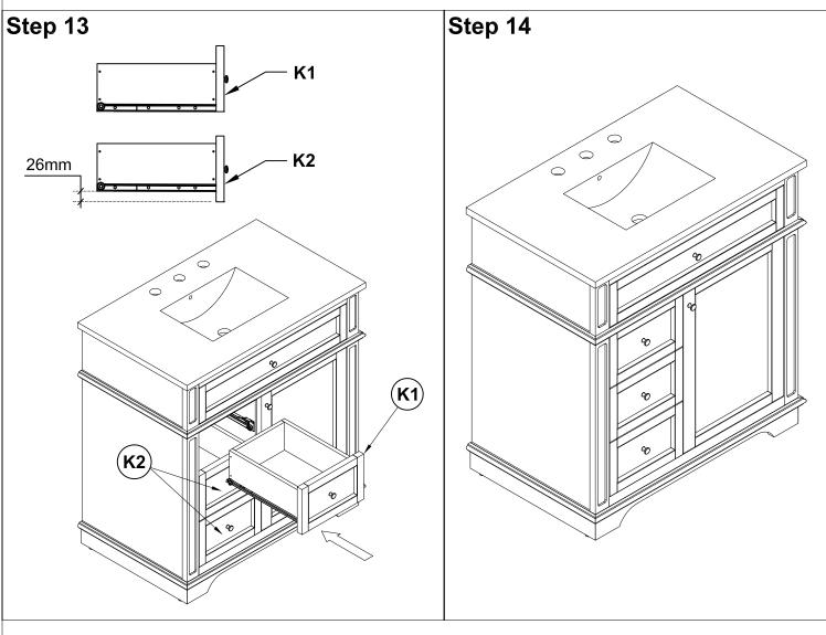
Put the drawer into the cabinet frame respectively like picture.
