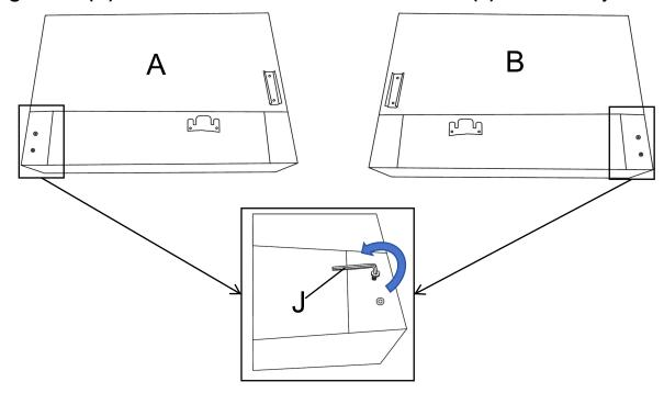
Step 2: Connect the Front **Seat Panel(C)** with **Left Arm(A)** and **Right Arm(B)** together and then secured with **Allen wrench(J)**
