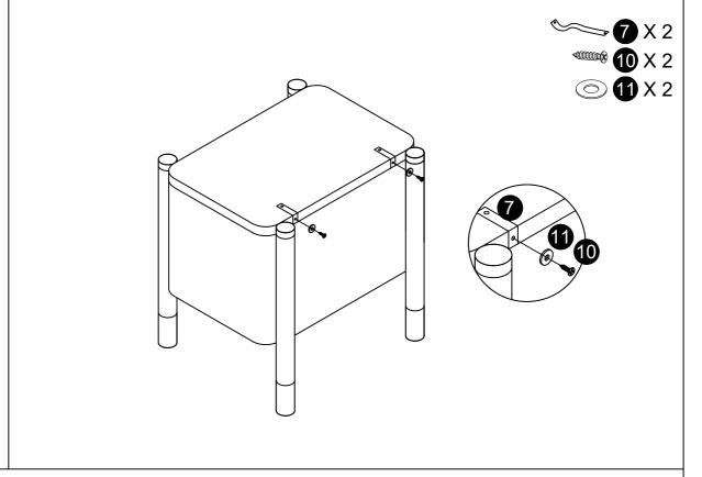
Align with the pre-drilled hole back side of the end table body (A) ,install the Anti-Tipping webbing (  $\bigcirc$  ) with short screw (  $\bigcirc$  ) and flat washer (  $\bigcirc$  ) .
