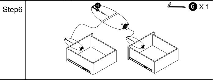
Unscrew the handle inside of the drawer using hex wrench(⑥).
