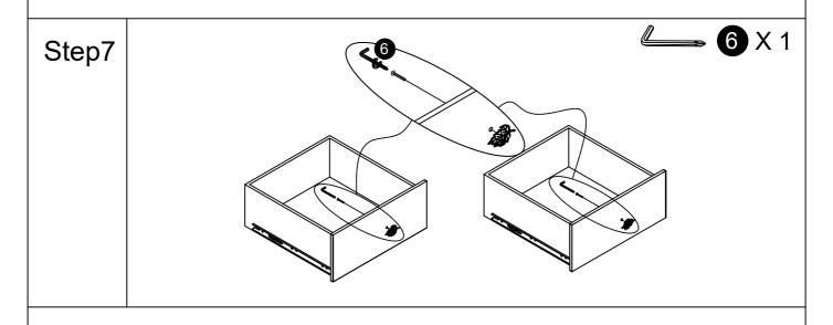
Screw the handle on the front of the drawer using hex wrench(⑥).
