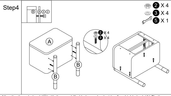
Align the threaded rod (①)with the pre-drilled holes on back side of end table body(A),Fix the leg (B) with hex nut (②) and flat washer (③) from inside of the end tablebody using flat open end wrench(⑤).
