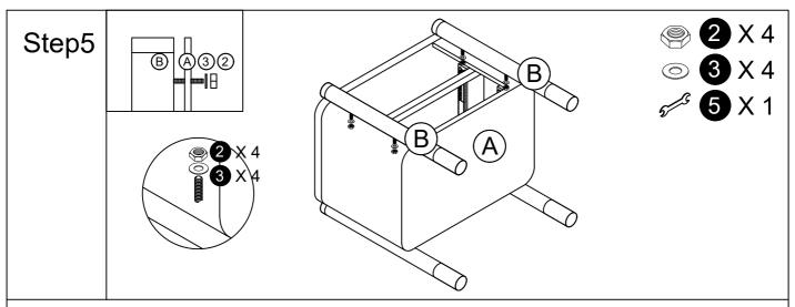
Align the threaded rod (①)with the pre-drilled holes on front side of end table body(A), Fix the leg (B) with hex nut (②) and flat washer (③) from inside of the end table body using flat open end wrench(⑤).
