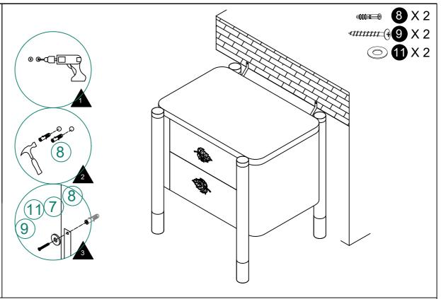
Drill holes on the wall, put expansion plugs (8) into the holes, align with the expansion plugs (8), install the Anti-Tipping webbing (7) with long screw (9) and flat washer (1).
