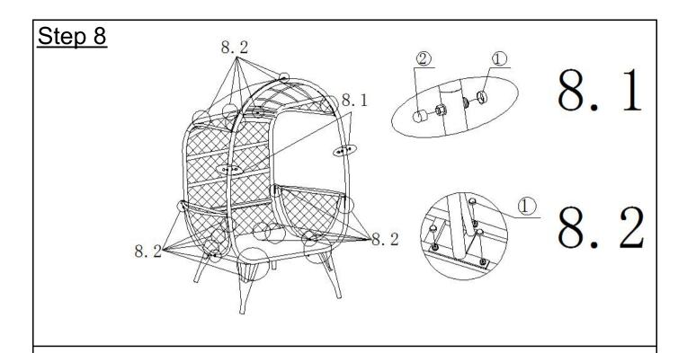
Cover all the Bolts and nuts with the Bolt Caps((1)) and the Nut Caps((2)) as shown in pictures 8.1 and 8.2.
