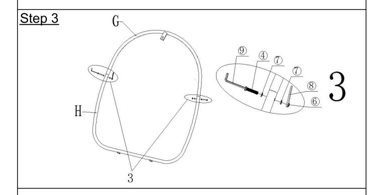
Attach the Basket Frame - Top(G) to the Basket Frame - Bottom (H) with the Allen Wrench(9) and Wrench (8), using Bolts (4), Washers(7) and Nuts (6) as shown in picture above. Do not fully tighten the bolts.
