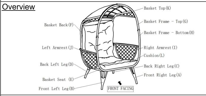
This Chair has multiple parts and may require up to some 30 minutes to assemble. To give you an overview of the Chair parts, the above picture is provided to help you put the various parts into perspective. Please read through the instructions below to familiarise yourself with the parts and steps before assembly.
