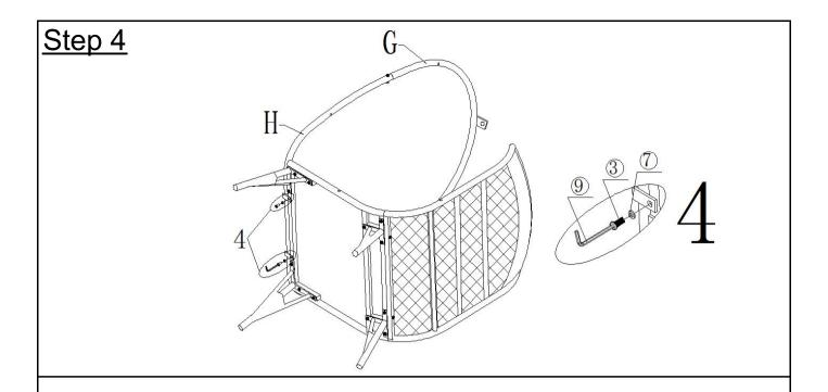
Attach the Basket Frame - Top(G) and the Basket Frame - Bottom (H) to the Basket Seat(E) with the Allen Wrench( $\mathfrak{D}$ ), using Bolts ( $\mathfrak{D}$ ) and Washers( $\mathfrak{D}$ ) as shown in the picture above. Do not fully tighten the bolts.
