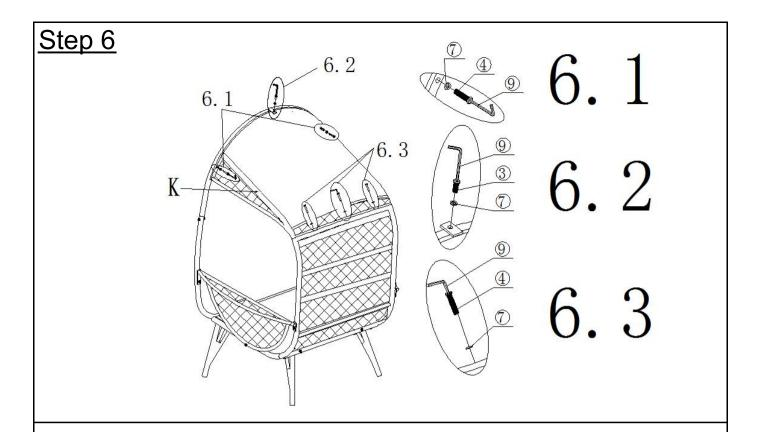
Attach the Basket Top(K) to the Basket Back(F) and the Basket Frame - Top (G) with the Allen Wrench( $\mathfrak{D}$ ), using Bolts( $\mathfrak{D}$ ), Bolts( $\mathfrak{D}$ ) and Washers( $\mathfrak{D}$ ) as shown in the picture above. Do not fully tighten the bolts.
