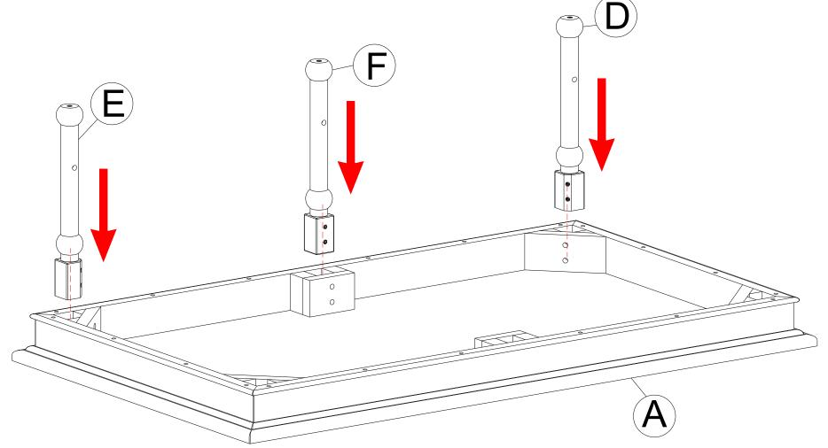
Put the Table Top (A) upside down on a soft surface. Position the First Leg (D), Second Leg (E), Middle Leg (F) to the Table Top (A) as shown above picture.
