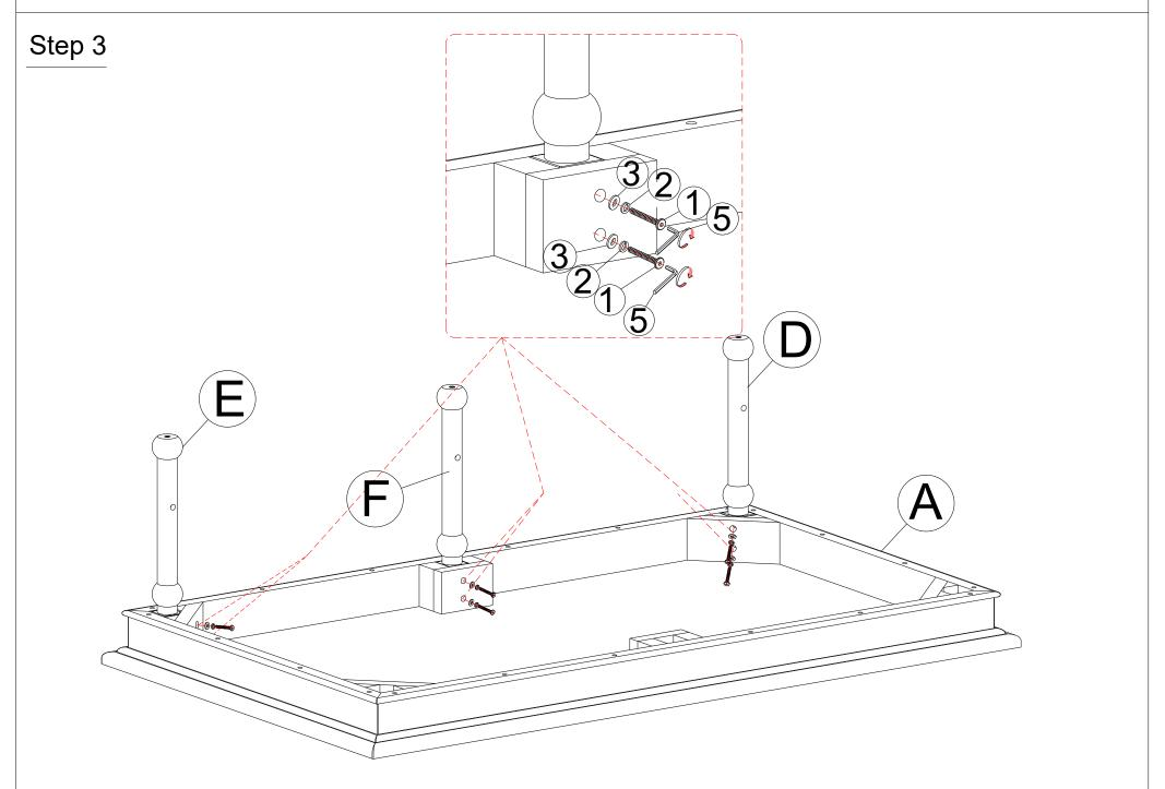
Attach the First Leg (D), Second Leg (E), Middle Leg (F) to the Table Top (A) using Bolt (1), Lock Washer (2), Flat Washer (3) and Allen Wrench (5) and tighten bolts.
