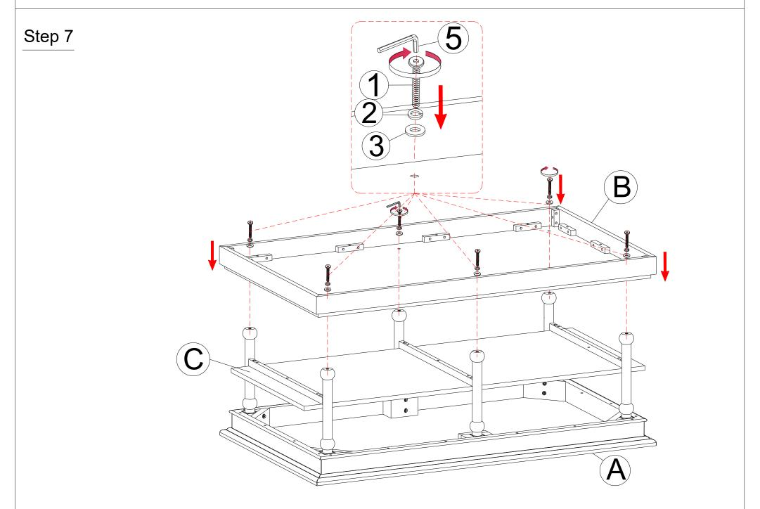
With assistance from your adult partner, attach Bottom Shelf (B) to the Legs using Bolt (1), Lock Washer (2), Flat Washer (3) and Allen Wrench (5) and tighten bolts as shown picture.
