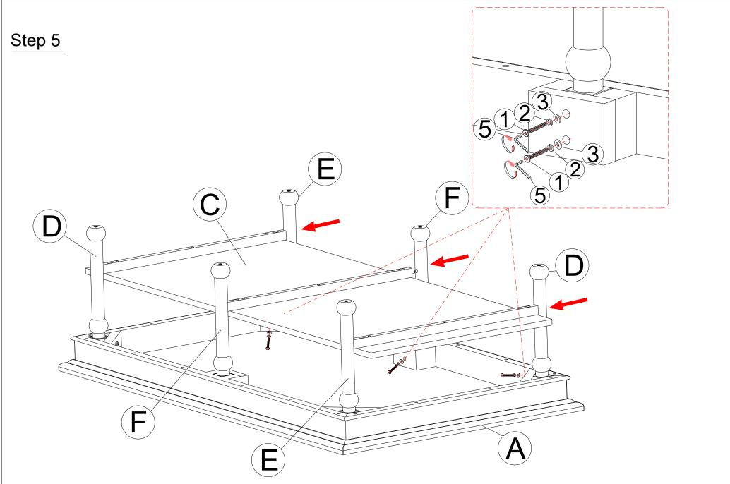
With assistance from your adult partner, repeat step 3 and step 4 to attach First Leg (D), Second Leg (E) and Middle Leg (F) to the Table Top (A) and Middle Shelf (C) using Bolt (1), Lock Washer (2), Flat Washer (3) and Allen Wrench (5) and tighten bolts as shown above picture.
