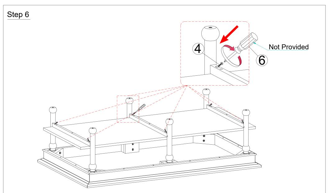
To secure the Middle Shelf (C) to the Legs using Screw (4) and Screw Driver (6) (not provided) and tighten Screw as picture.
