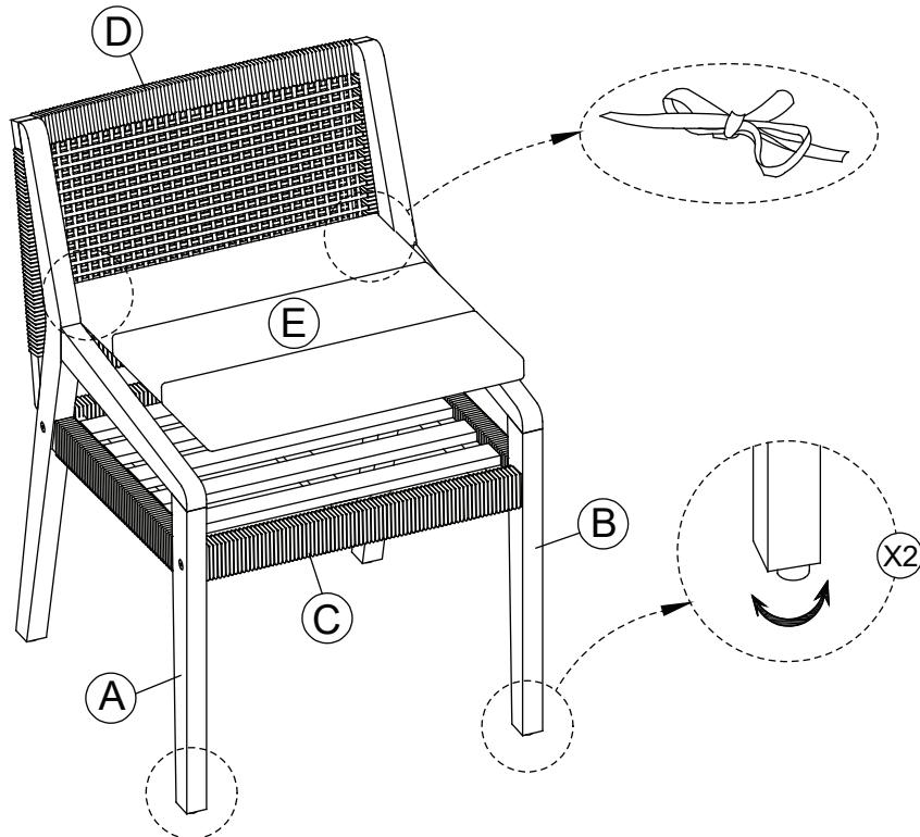
Place the Seat Cushion (E) on the Chair as shown above. Tight Cushion ropes directly to the chair frame. Turn the product upright and adjust the levelers at the bottom of the legs (if needed) to balance the Chair.
