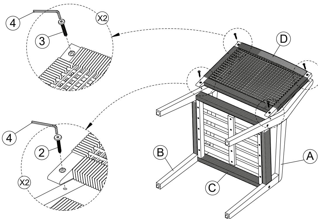
Attach Back Panel (D) into assembled frame from Step (2) by using Screw (2) and Bolt (3) as shown in the above picture.
