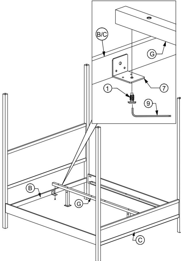
With the help of another adult ,attach Center Support (G) to Headboard Support (B) and Footboard Panel (C) using JCBC Bolts (①) with Allen Wrench (⑨) as indicated on the diagram above.
