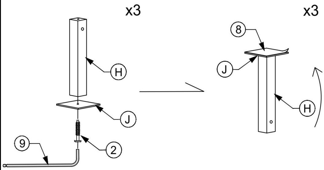
Attach Support Post Pad (J) to Support Posts (H) using JCBC Bolts (2) with Allen Wrench (9). Where indicated on the diagram above. Using sticker Eva Pad (8) stick to Support Post Pad (J) as indicated on the diagram above.
