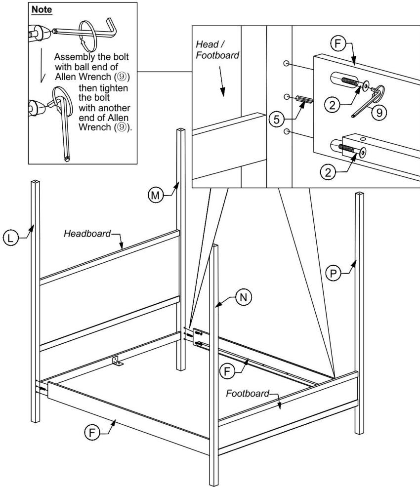
With the help of another adult ,attach Side Panels (F) to Headboard Post Left (L), Headboard Post Right (M), Footboard Post Left (N) and Footboard Post Right (P) using JCBC Bolts (②) and Wood Dowels (⑤) with Allen Wrench (⑨) as indicated on the diagram above.
