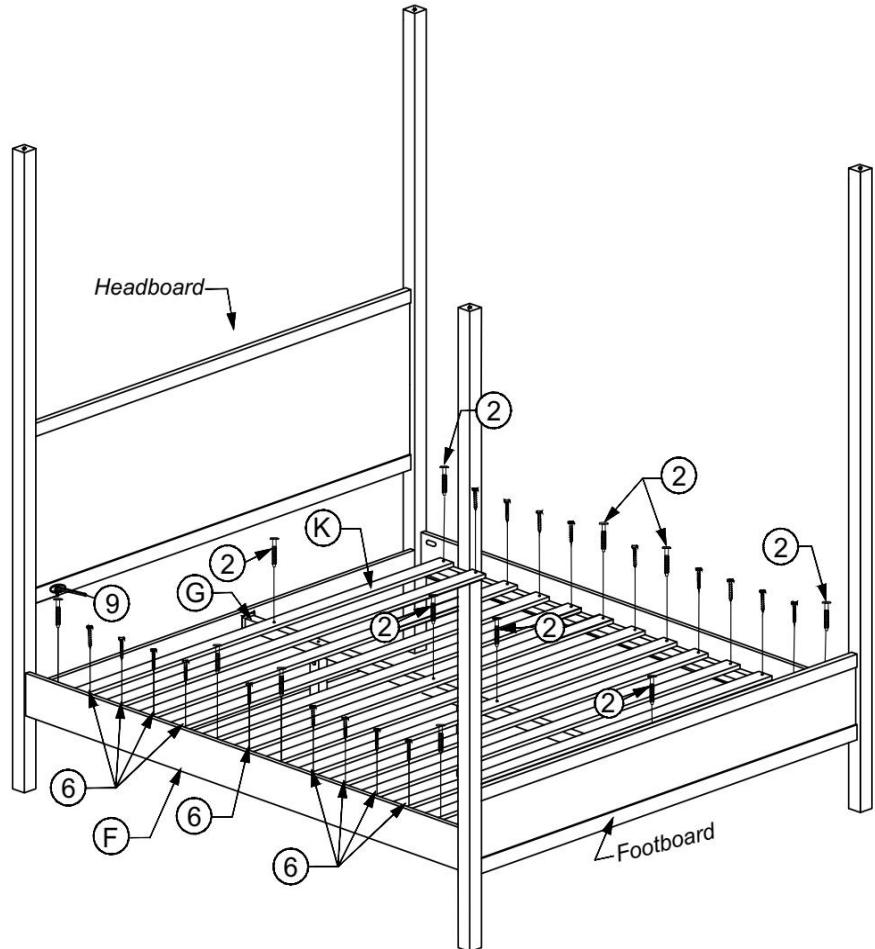
With the help of another adult ,attach Bed Slats (K) to Side Panels (F) and Center Support (G) using JCBC Bolts (②) and CSK Screw (⑥)with Allen Wrench (⑨) as indicated on the diagram above.
