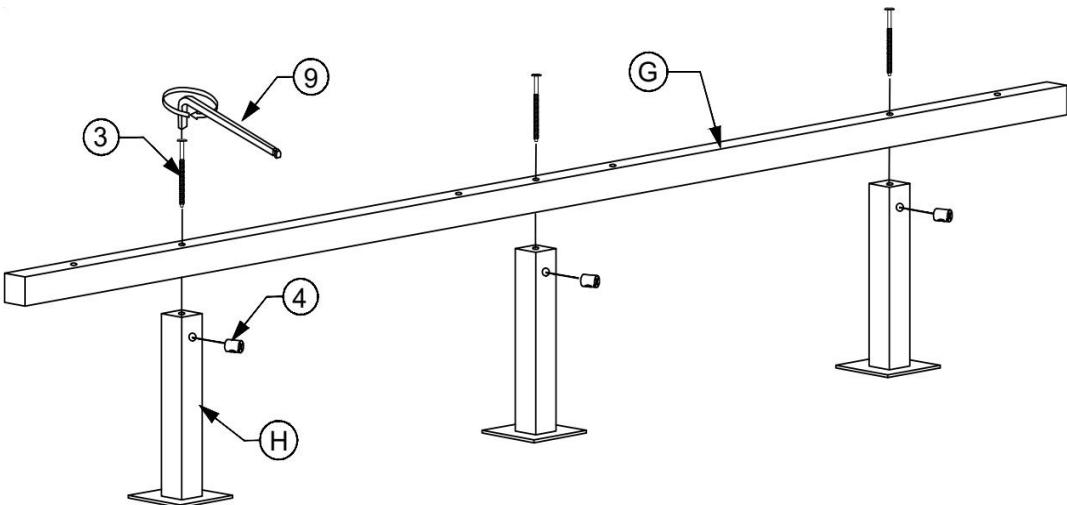
Attach Center Support (G) to Support Posts (H) using JCBC Bolts (③) and B/Nut (④) with Allen Wrench (⑨) as indicated on the diagram above.
