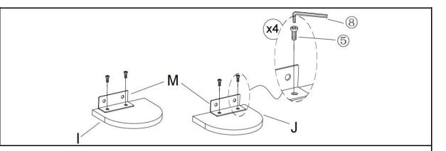
Attached Small L-shaped Iron (M) to Shelves-I(I) and Shelves-J(J) by using Bolt (5) and Allen Wrench (8), as pictured above.
