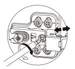
You can adjust one or both hinges on each door, depending on how much correction it needs. If the door seems to be tilting down to the right, turn the side-to-side screw on the top hinge so the hinge pulls closer to the side of the cabinet box, moving the top of the door to the left.
