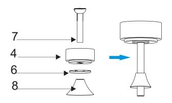
4. Loosen two set screws on the downrod support and then place the downrod into the downrod support.
