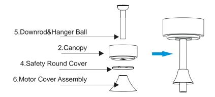
4. Loosen two set screws on the downrod support and then place the downrod into the downrod support.
