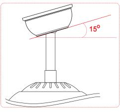
2. For wood ceiling, secure the mounting bracket to the ceiling that is capable of carrying a load of at least 100lbs (45kgs) with two long mounting screws and washers provided. Be sure at least 0.12"(30mm) of the screw is threaded into the support.
