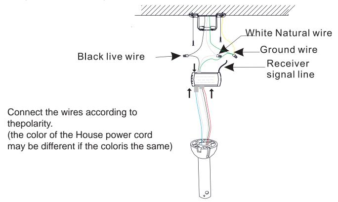
Correctly link the light wire, motor wire, and neutral wire and live wire according to the guidelines on the right.
