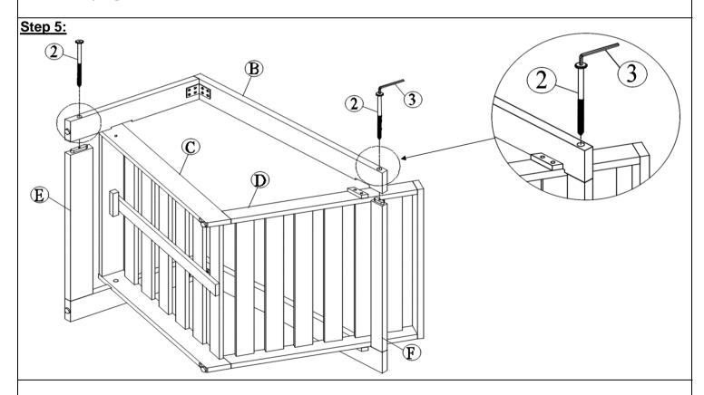
With the help of your adult partner, attach the Right Arm Panel (B) to the assembled part in Step 4 and then secure by using Screws (2) and Allen Wrench (3).
