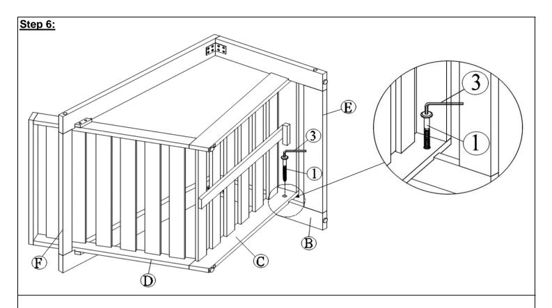
With the help of your adult partner, turn the assembled part in Step 5 to the opposite side and then secure the Right Arm Panel (B) to the Seat Panel (C) by using Screws (1), and Allen Wrench (3). **Do not fully tighten the Screws.**
