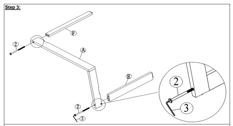
With the help of your adult partner, place Left Arm Panel (A), Front Support Bar (E) and Back Support Bar (F) the stand up as shown in picture onto a clean, soft surface to avoid any scratches or damages to the product.
