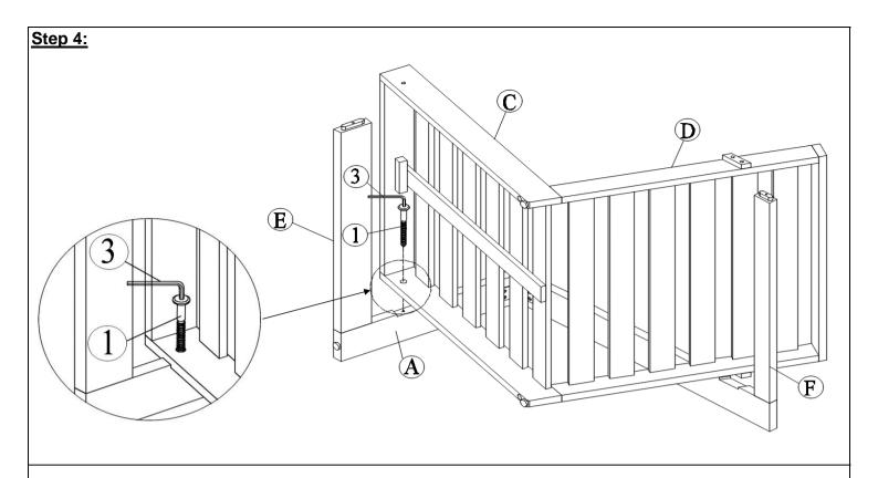
With the help of your adult partner, attach the assembled part in Step 2 to the assembled part in Step 3 and then secure by using Screws (1) and Allen Wrench (3) as shown above.
