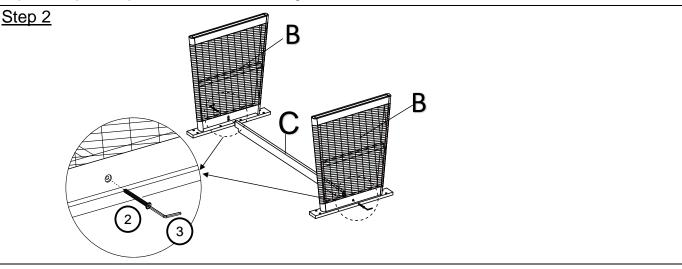
Place the Leg Panel (B) laid down as shown in the picture above onto a clean, soft surface to avoid any scratches or damage to the product. With assistance from your adult partner(s)
