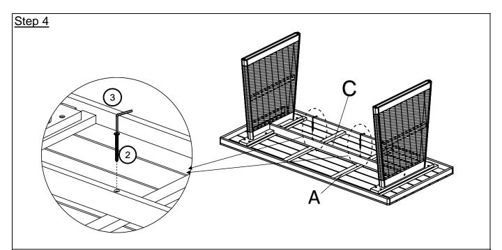
Flip the Table Top (A) (bottom-side up) and place it on a clean, soft surface to avoid any scratches or damage to the product.
