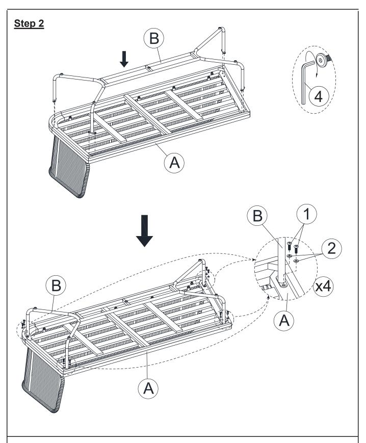
With assistance from your adult partner, place the seat frame (A) facedowwn onto a clean, non marring surface, then attach the Leg Frame (B) to the Seat Frame (A) using the Bolts (1), Washers (2) and the Allen Wrench (3).
