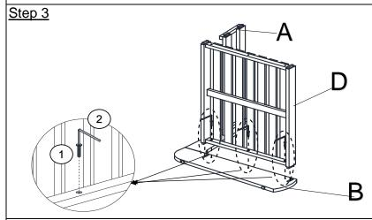
Place the Right Leg Panel(B) facedown onto a clean, non-marring surface. Attach Seat Panel(D) to Right Leg Panel(B) using  $Bolts(\widehat{\ 1})$  with Allen Wrench ( $\widehat{\ 2}$ ), as show above. **Do not fully tighten the Bolts.**
