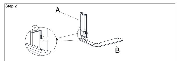
Place the Right Leg Panel(B) facedown onto a clean, non-marring surface. Insert the dowels of Backrest Panel(A) into the mountings in the Right Leg Panel(B). Attach Backrest Panel(A) to Right Leg Panel(B) using Bolt(1) with Allen Wrench (2), as show above. **Do not fully tighten the Bolts.**
