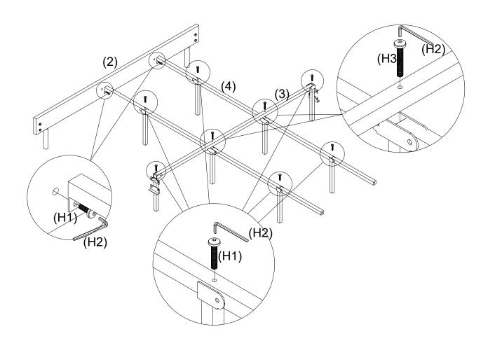
Step 3 Lay the headboard (1) flat on the clean floor, put the headboard support frame (8)on it, and tighten it with (H1) and (H2)
