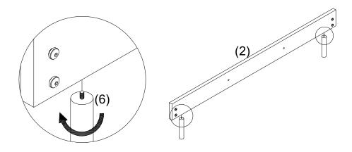
Step2 Please install part (2) and part (3) on part (4), tighten the bolts (H1)
