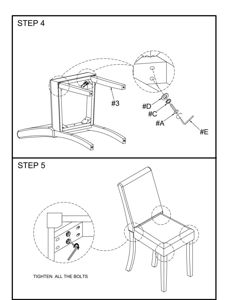
Do not tighten screws until completely assembled.
