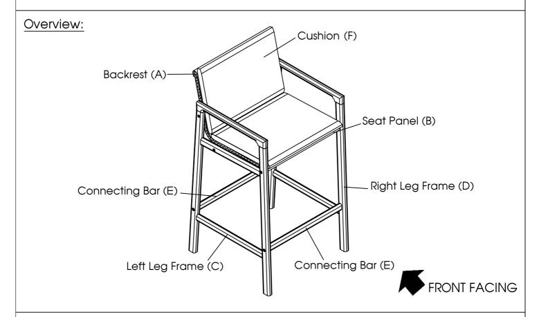
This Chair has multiple parts and may require up to 15 minutes to assemble. To give you an overview of the Chair parts, the above picture is to help you put the various parts into perspective. Please read through the instructions below to familiarise yourself with the parts and steps before assembly.
