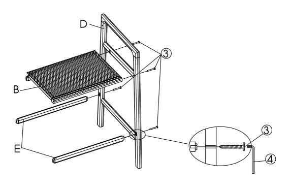
With the help of your adult partner, fix the 02 Connecting Bar (E), Seat Panel (B) with the Right Leg Frame (D) by using 04 screws (3) by Allen Wrench (4). Do not fully tighten the screws.
