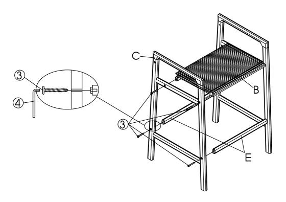
Fix the Left Leg Frame (C) to the Seat Panel (B) and 02 Connecting Bar(E) secure by using screws (3) and Allen Wrench (4). Do not fully tighten the screws.
