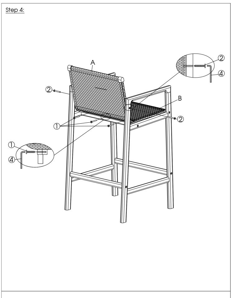
Fix the backrest (A) with Seat Panel (B) by using the Screws (1) by Allen Wrench (4) then fix the backrest with 02 leg, secure by using screws (2) and Allen Wrench (4). Do not fully tighten the screws.
