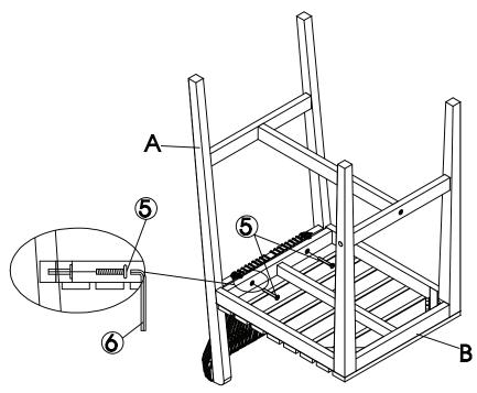
Use the bolts (5) flx the Seat Panel (B) with backrest (A) by using the Allen Wrench. Do not fully tighten the screws.
