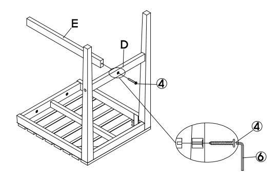
Fix the cross bar (E) with the front connecting bar (D) by using 01 screws (4) by Allen Wrench (6). Do not fully tighten the screws.
