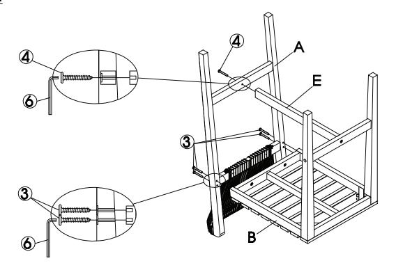
Fix the backrest (A) to the Seat Panel (B) and secure by using screws (3) and Allen Wrench (6) and fix the backrest together with the cross bar (E) by screw (4) and Allen Wrench. Do not fully tighten the screws.
