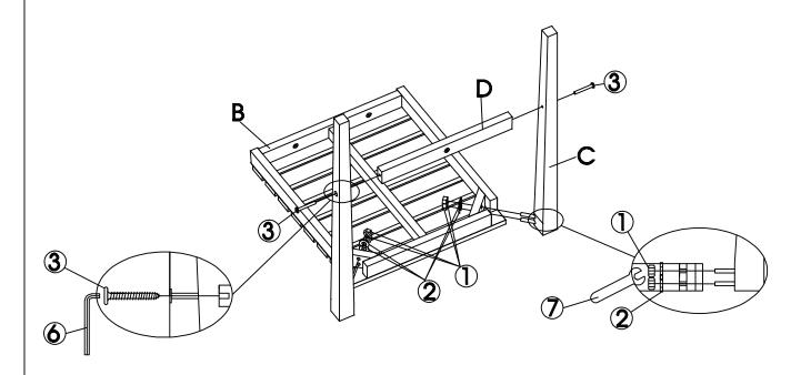
With the help of your adult partner, place the Seat Panel (B) facing down and then add the Front Leg (C) to the Seat Panel (B) and secure by using Nuts (1) + washer (2) by Wrench after that fix the front connecting bar (D) with 02 screws (3) by Allen Wrench (6). Do not fully tighten the screws.
