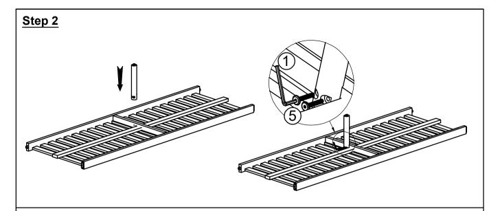
With the help your adult partners, place Seat Panel (D) as above picture. Attach Support Leg (G) to Seat Panel (D) by using 2 Bolts ( $\mathfrak{S}$ ) and Allen Wrench( $\mathfrak{D}$ ). **Do not fully tighten the Bolts.**
