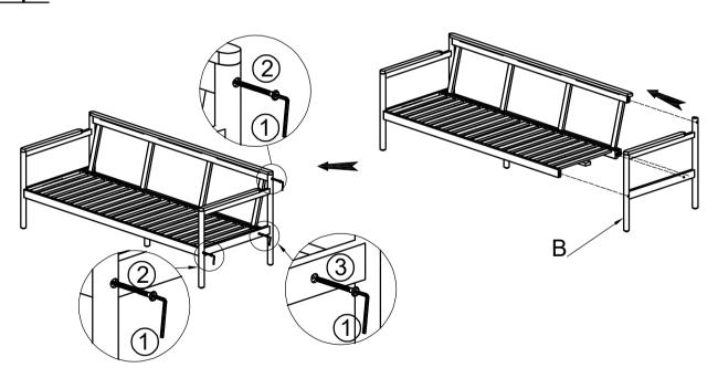
Attach Right Leg Panel (B) to Seat Panel (D) and Backrest Panel (C) by using Screws (2)+(3) and Allen Wrench (1).
