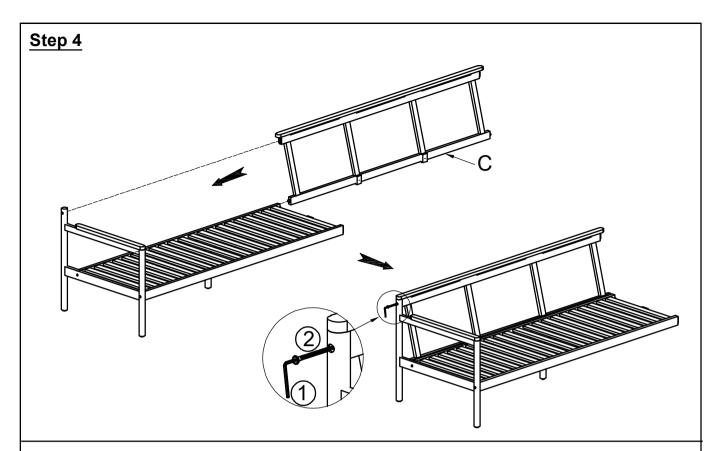
Attach Backrest Panel (C) to Left Leg Panel (A) by using Screw (②) and Allen Wrench(①).
