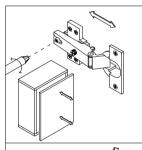
If the hinge holes are notaligned, you can tryadjusting the front and rear hinges.
