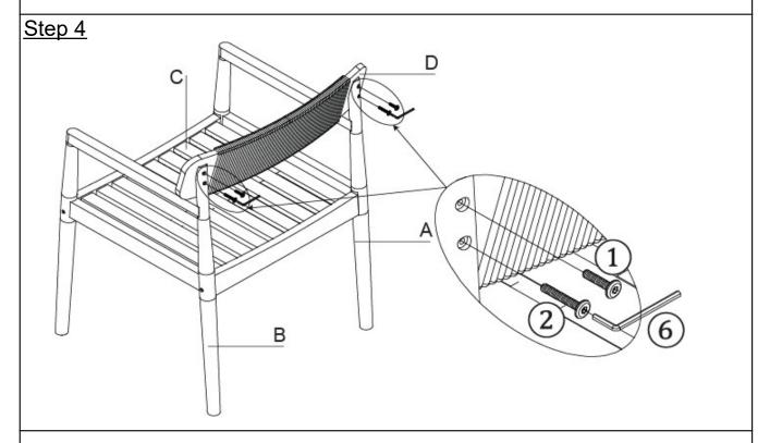
Attach the assembled parts from Step 3 to the Backrest Panel (D) using Bolts (1), Bolts (2) with the Allen Wrench (6) as shown above. **Do not fully tighten the Bolts.**
