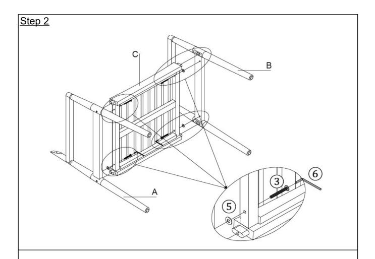
Place the Left Leg Panel (A), Right Leg Panel (B), Seat Panel (C) facedown on a clean, non-marring surface as shown above.
