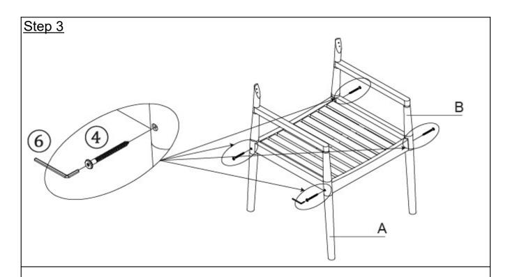
Secure the Left Leg Panel (A), Right Leg Panel (B) and Seat Panel (C) using Screw (4) with the Allen Wrench (6) as shown above. **Do not fully tighten the Screws.**
