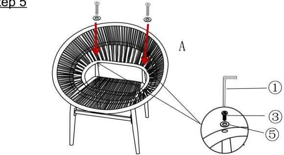
Use Bolts (③) and Washers (⑤) with Allen Wrench (①) to connect the Seat Part (A) and Right Leg (B) and Left Leg (C) as shown above.
