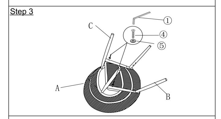
Use Bolts (4) and Washers (5) with Allen Wrench (1) to attach the back part.
