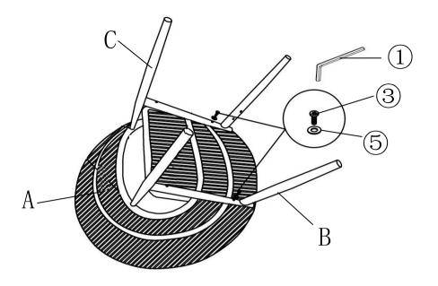
Attach the Left Leg (C) and the Right Leg (B) to the Seat Part (A) using Bolts (③) and Washers (⑤) with Allen Wrench (①) as shown above.
