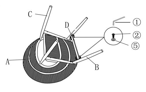
Attach the Legs Connection (D) to Left and Right Leg (C & B ) using Bolts (2) and Washers (5) with Allen Wrench(1) as shown above.
