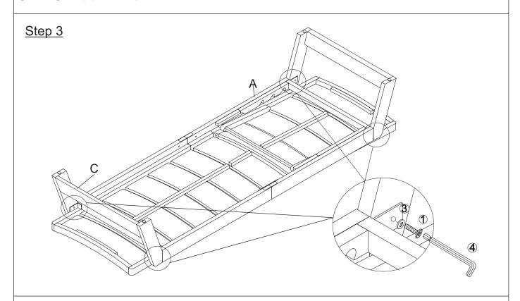
Attach the Leg Panel (C) to the Foldable Seat Panel (A) using Bolt (1) and Washer (3) with Allen Wrench (4) as shown in the picture.
