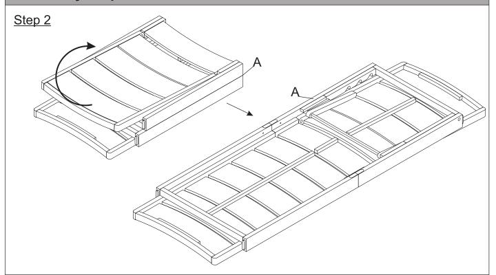
Unfold the Foldable Seat Panel(A) as indicated by the arrows.
