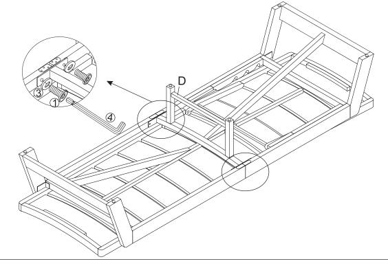
Attach Middle Leg (D) to Foldable Seat Panel (A) using Bolts (1) and Washers (3) with Allen Wrench (4) as show in the picture.
