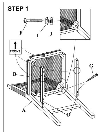
Attach the seat (B) to backrest (A). Ensure the seat (B) align to the matching holes. Insert the small washer (J), spring washer (I) and 2" bolt (F) to the holes as shown in the diagram above. Adjust the bolts to the right position before screwing.
