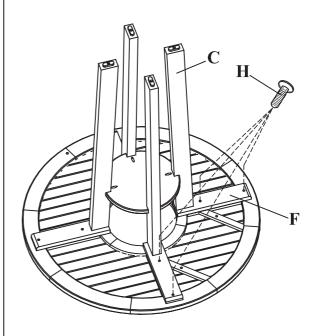
Attach two set leg (C) and leg bar (F) to the previous assembly. Secure using 1" bolts (H).
