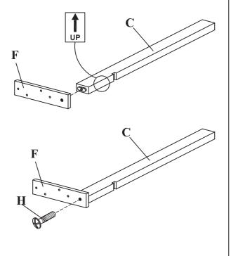
Install Leg bar (F) to leg (C), secure using 1" bolts (H). Pay attention to the position of the notch on the leg to the leg bar (F).
