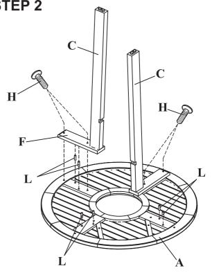
Insert dowel (L) into the hole on the underside table top (A), then attach two set of leg (C) and leg bar (F) assemblies from step 1 to the table top (A) and secure using 1" bolts (H) as shown.
