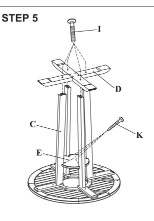
Attach base frame (D) to the leg (C), secure using 1 3/4" bolt (I) and secure shelf (E) using 1 1/4" screw (K), as shown.
