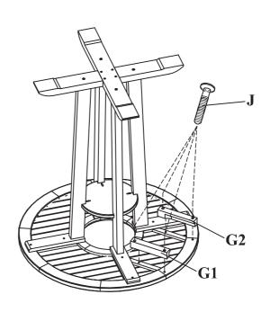
Attach right and left rail (G1&G2) to the table top (A), secure using 2" bolts (J).
