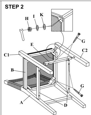
Attach the right and left leg (C1&C2) into the seat (B) and side aprons (D), secure using big washer (K), spring washer (I), nut (H) and 2 1/2" screw (G). As shown. Next attach front apron (E) to both front legs (C1&C2), secure using 2 1/2" screws.
