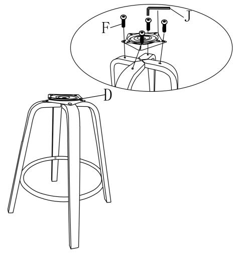
Finally tighten all screws to a depth of 100%.
